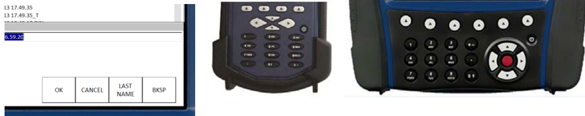
Figure 10: All Modules – Storing of last entered filename respectively recall within a firmware Module via function key „LAST NAME“ (left) / comparison of VT-80/VP-80 key pad with function keys, alpha numeric keys and Cursor cross with Fire Key for quick navigation (right)
