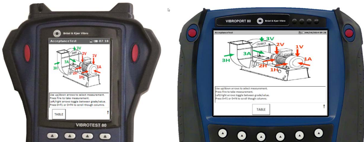
Figure 9: Module 11 Acceptance – Displays of user defined integrated machine picture *.bmp for better orientation (VT-80 left / VP-80 right)
