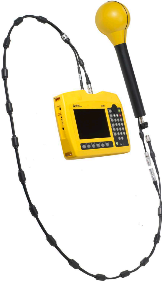
Figure 3: Connecting the SRM-3006 to an antenna using a cable.
