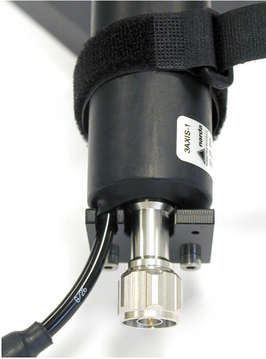
Figure 6: Cable and N connector in guideway
