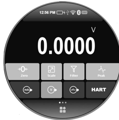
Figure 6 Electrical signal measurement function
