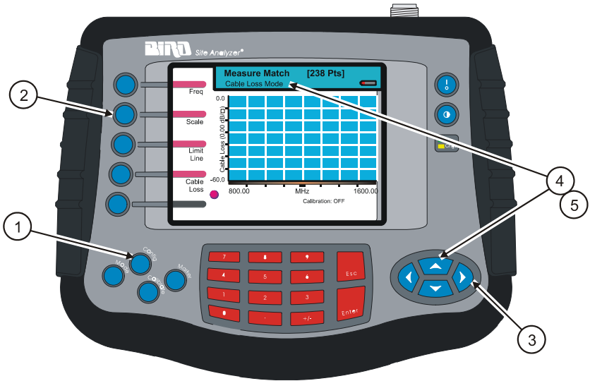
Figure 18 Set Up for Cable Loss Measurement
