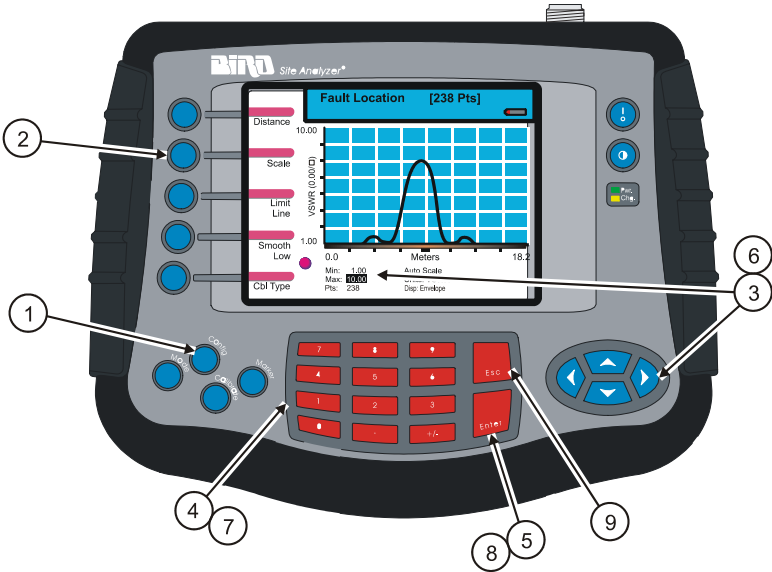
Figure 28 Setting Fault Location Scale Limits Manually
