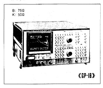
The MS420B/K Network/Spectrum Analyzer is suitable for total evaluation of electronic devices, circuits, and elements. It can analyze magnitude, phase, delay time, levels and spectrum, and frequencies of signals. The MS420B/K also has a built-in test-signal source and CRT display.
