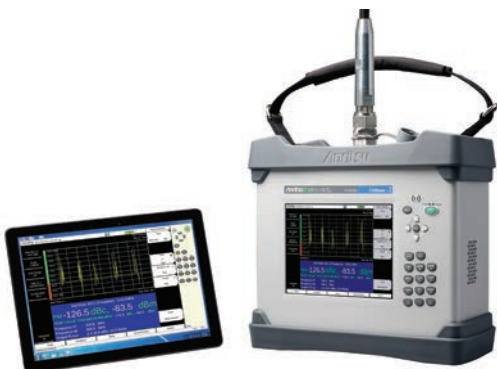
Remote Access Tool for Tower Top Testing
