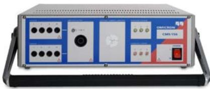
CMS 156 amplifier units can be used in combination with any CMC test set or in conjunction with digital real time power system network simulators. The outputs are galvanically separated from the inputs as well as from ground and are used independently or in addition to those of the CMC test sets. The connection to a CMC test set is made by a control cable at the back of the units.
