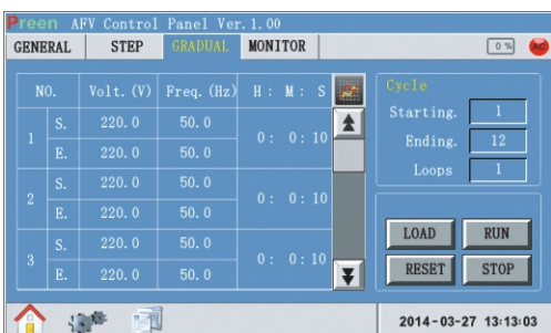
Voltage and Frequency Setting Interface at Gradual Change Mode
