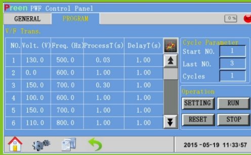
Voltage and Frequency Setting Interface at Step Change Mode
