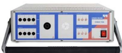
CMA 156 amplifier units can be used in combination with any CMC test set or in conjunction with digital real time power system network simulators. The outputs are galvanically separated from the inputs as well as from ground and are used independently or in addition to those of the CMC test sets.
