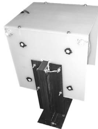
60KV Impulse Isolation Transformer. Less than 20PF primary to secondary or to ground. 115/230V to 115/230V, 50 volt amps.
