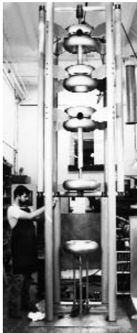
GD350-DOUBLETHROW 350KV PK TEST 1500 AMPS, 30KHz
