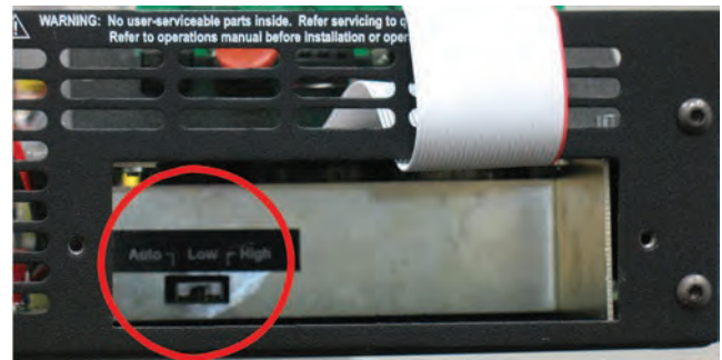
Figure 5.12 – Bi-Level Power Switch Location
