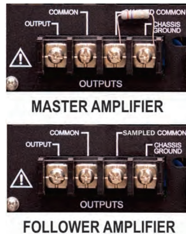
Figure 6.29 – Remove the 2.7-ohm resistor from Follower amplifiers
