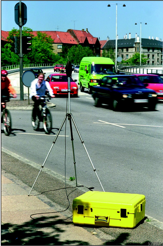
Fig. 4 Outdoor Gear Type 3592 and Outdoor Microphone Kit UA 1404
