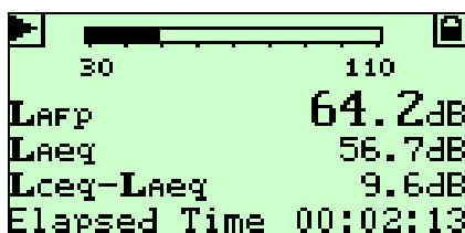
Fig. 3 Sample screen from Enhanced SLM Software BZ 7125. Note that A- and C- weighted values are available simultaneously. Mediator's dual RMS detectors simultaneously compute F, S and I time constants in parallel
