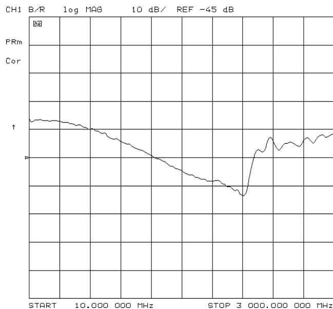
Figure 2-35 Example Mixer LO to RF Isolation Measurement
