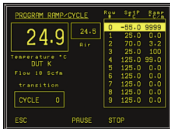
Set up to 12 temperature tests sets in Program Mode, while DUT Control monitors device temperature directly.
