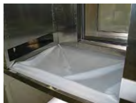
Flexible diaphragm floor for use with vibration shaker.
