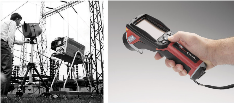
Figure 16.1 LEFT: ThermoVision® Model 661 from 1969. The camera weighed approximately 25 kg (55 lb.), the oscilloscope 20 kg (44 lb.), and the tripod 15 kg (33 lb.). The operator also needed a 220 VAC generator set, and a 10 L (2.6 US gallon) jar with liquid nitrogen. To the left of the oscilloscope the Polaroid attachment (6 kg/13 lb.) can be seen. RIGHT: InfraCAM from 2006. Weight: 0.55 kg (1.21 lb.), including the battery
