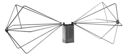
The assembly design of the Model 3109 provides for easy storage and portability. The standard biconical elements are made from welded aluminum. The 4-to-1 ratio balun network is fabricated from TFE thermoplastics and specially machined brass and aluminum support and contact parts. The bifilar inductors of the balun are wound in precision machined cuts to provide high barrier insulation between windings while simultaneously giving good coupling between bifilar windings.
