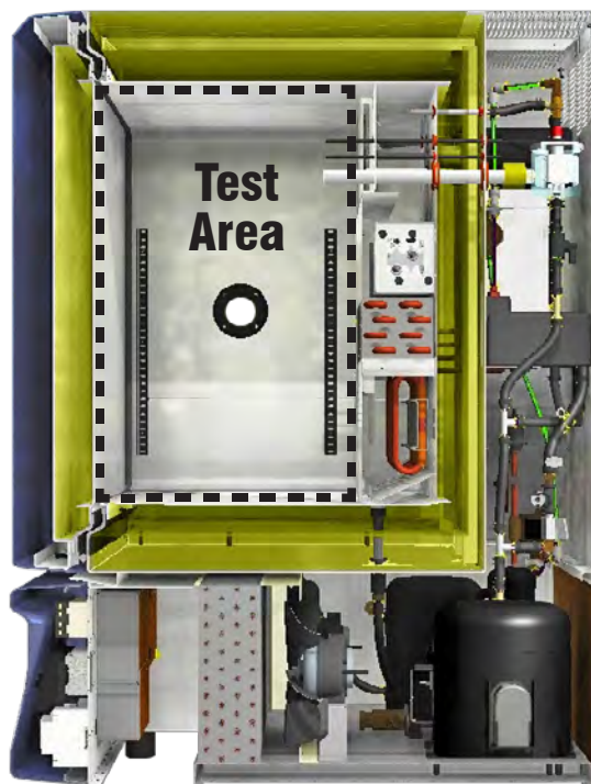
The chamber's fan continuously circulates conditioned air from the test area to the plenum (to the right of the test area), where the heaters, cooling coil, and humidity inlet are located. (BTX-475 model shown).
