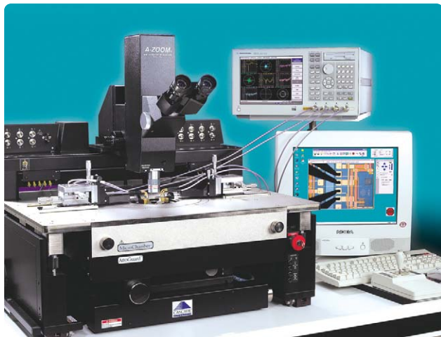
Agilent ENA RF network analyzer and Cascade Summit 12000 Probing System
