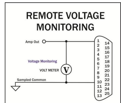
Figure 5.4 - Remote Voltage Monitoring Schematic
