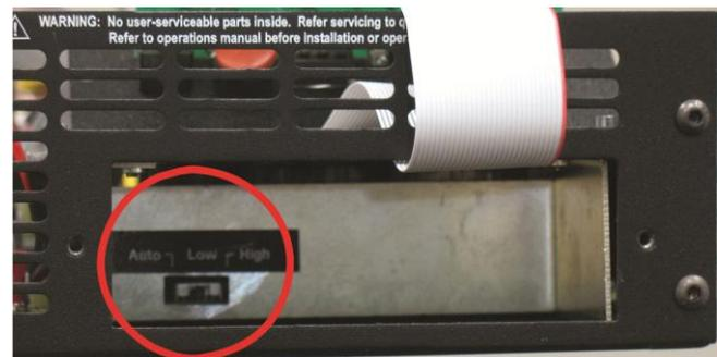
**Figure 4.14– Bi-Level Power Switch Location**
