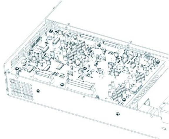
Figure 4.2 – Main Board Location inside Access Panel
