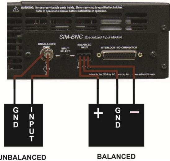
Figure 2.5 – Wiring for Unbalanced or Balanced Input Connector
