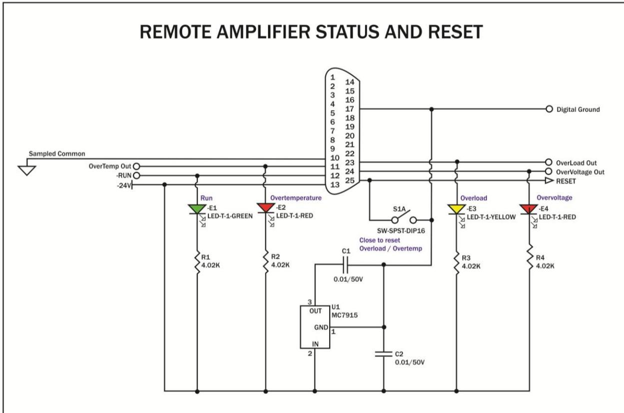
Figure 5.3 – Remote Status and Reset Schematic
