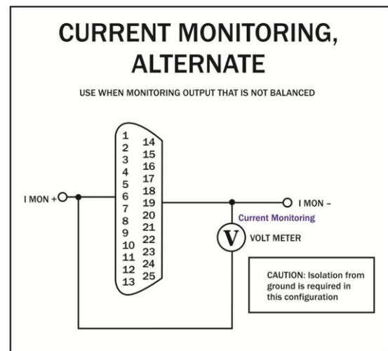
Figure 5.6 – Remote Current Monitoring Schematic, Alternate Method
