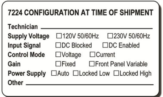
Figure 2.7 – Sample of Configuration Settings Label
