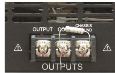
Figure 2.3 – Close-up of the Output Terminals
