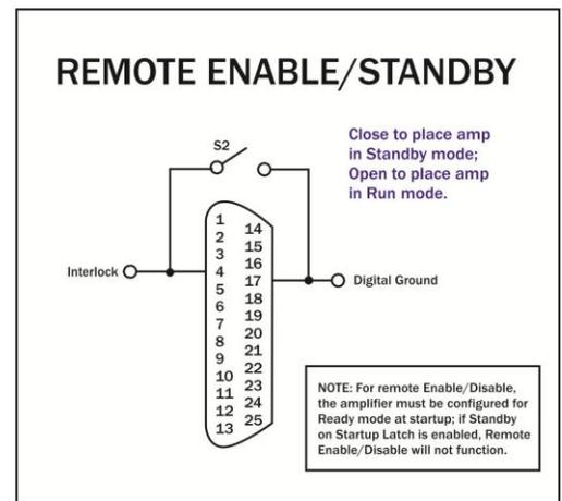
**Figure 5.2 – Remote Enable/Standby**
