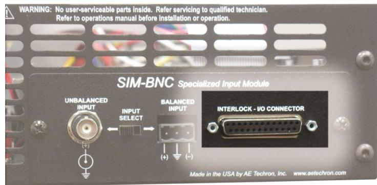
Figure 8.3 - Interlock I/O Connector
