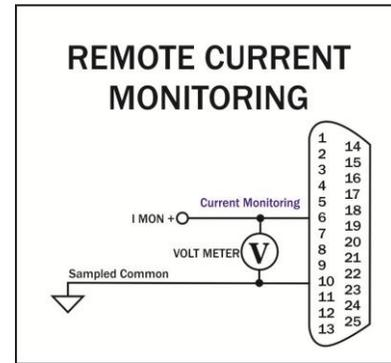
Figure 5.5 – Remote Current Monitoring Schematic
