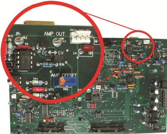
Figure 4.5 - Controlled Voltage / Controlled Current Setting
