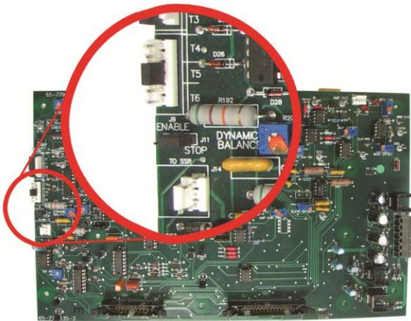
Figure 4.7 - Ready Mode/Standby Mode Power Up Setting
