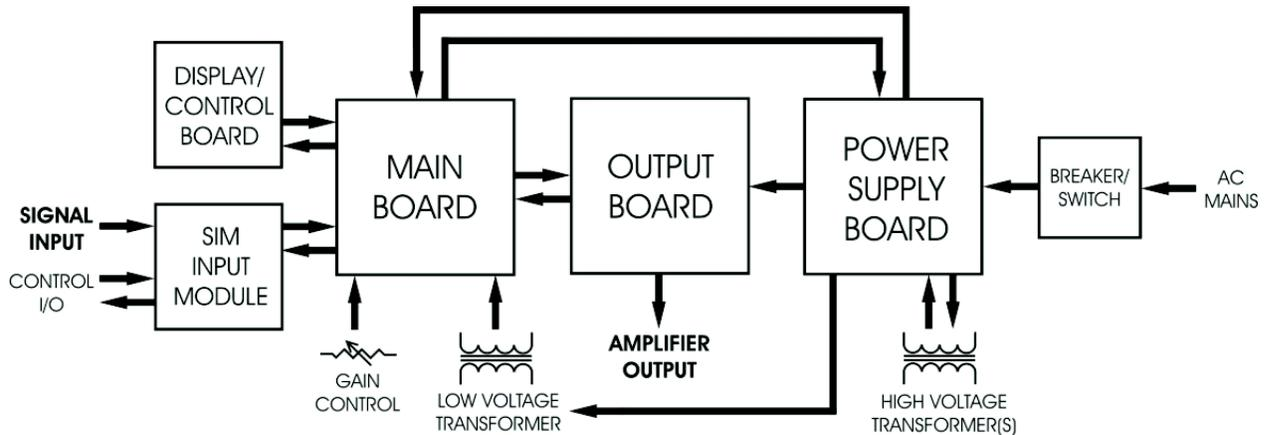
Figure 6.1- Board-Level Functional Block Diagram
