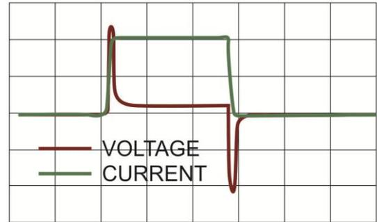
Figure 5.8 – Input to Output Comparison, Controlled-Current Operation
