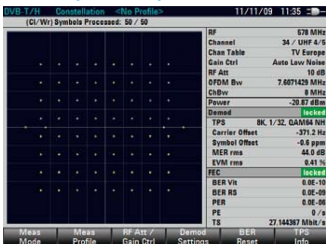
Constellation diagram of a DVB-T signal with excellent MER.
