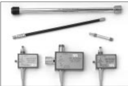
Offset SWR Autotesters and Precision Airlines measure high return loss values from 20 dB to 60 dB.
