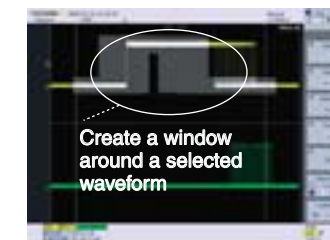
Waveform window search Select a waveform in History Memory and create a window around the waveform by moving up/down/left/right from the waveform. Search for waveforms that fall inside or outside the window.
