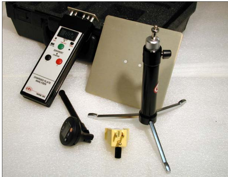
Figure 2-2: Model 216 Charged Plate Monitor Kit
