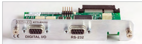
KTTI-RS232 RS-232 interface with 6 digital I/O ports.
