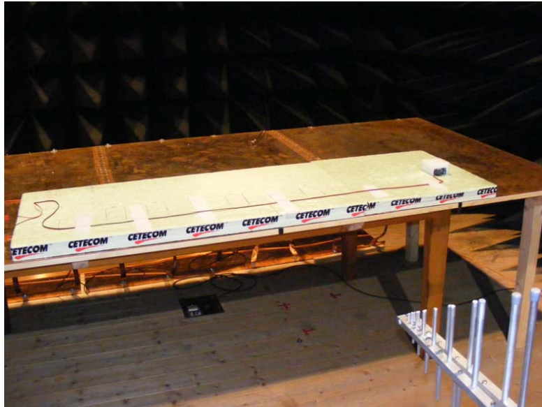
Photo 2: Emission Stripline 500 kHz - 1000 MHz
