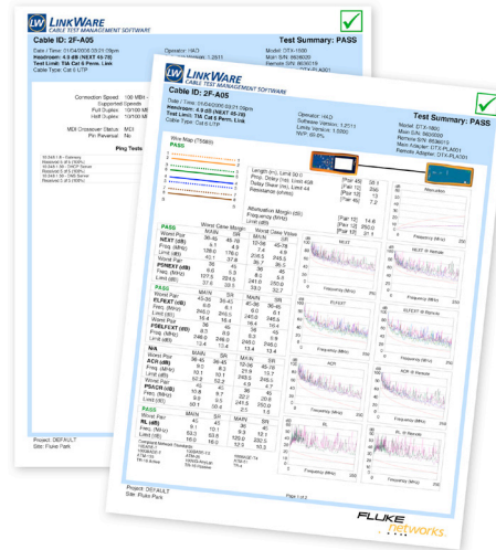
Document all the network tests executed as an integrated part of the cable certification documentation provided by LinkWare.
