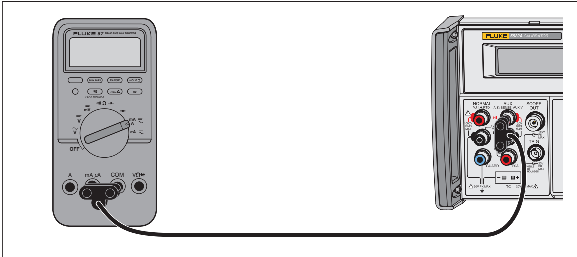
Figure 4-8. UUT Connection: DC Current/AC Current
