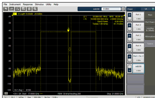
Improved flatness and lower noise floor in the notch after signal correction
