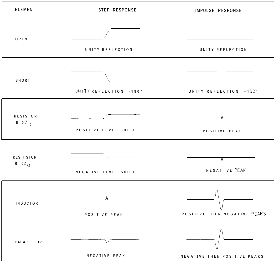
Figure 6-66. Simulated Low Pass Step and Impulse Response Waveforms (Real Format)
