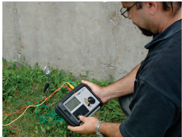
Model DET3TC shown performing the classic fall-of-potential test method.
