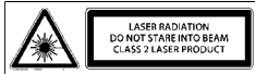
Figure 9.4 Wavelength: 635 nm. Max. output power: 1 mW. This product complies with 21 CFR 1040.10 and 1040.11 except for deviations pursuant to Laser Notice No. 50, dated July 26th, 2001
