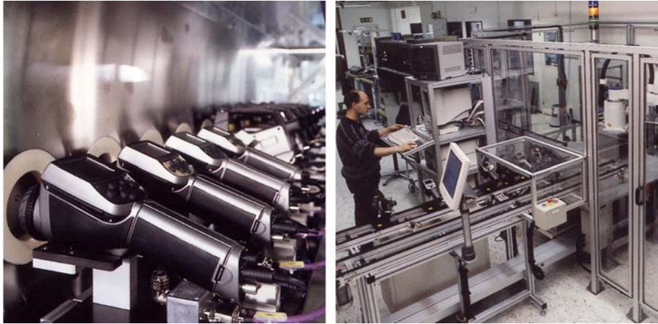
Figure 3.6 LEFT: Testing of IR cameras in the climatic chamber; RIGHT: Robot for camera testing and calibration
