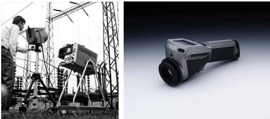
Figure 3.3 LEFT: FLIR Systems Thermovision® Model 661. The photo is taken on May 30th, 1969 at the distribution plant near Beckomberga, in Stockholm, Sweden. The camera weighed approx. 25 kg (55 lb), the oscilloscope 20 kg (44 lb), the tripod 15 kg (33 lb). The operator also needed a 220 VAC generator set, and a 10 L (2.6 US gallon) jar with liquid nitrogen. To the left of the oscilloscope the Polaroid attachment (6 kg/13 lb) can be seen. RIGHT: FLIR Systems ThermoCAM Model E2 from 2002 – weight: 0.7 kg (1.54 lb), including battery.
