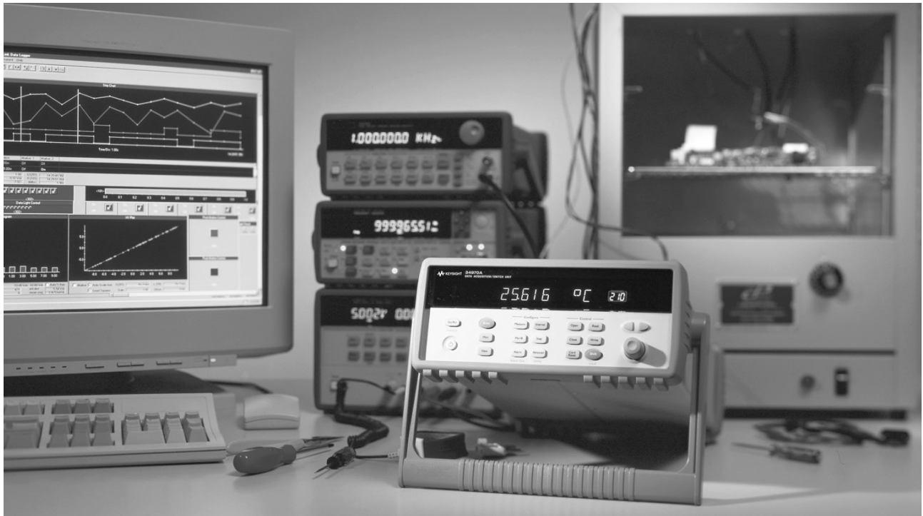
Compact 60-channel data acquisition system
