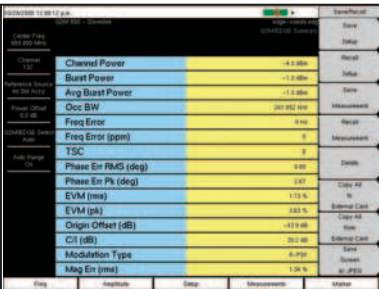
Option 41 provides a quick, table view of critical test parameters, including channel power, occupied bandwidth, phase error and EVM.
