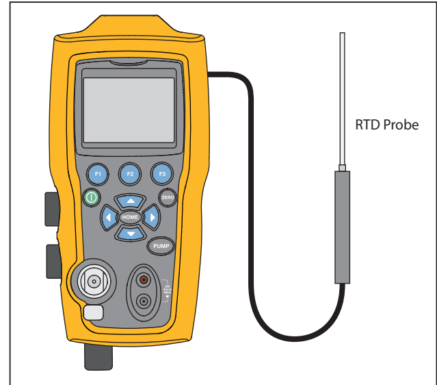
Figure 7. Temperature Measurement with RTD Probe
