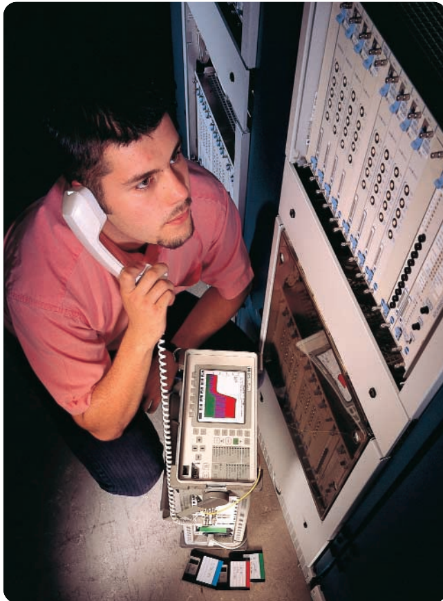
Portable SONET/SDH test sets measure optical rates to 2.5 Gb/s.
