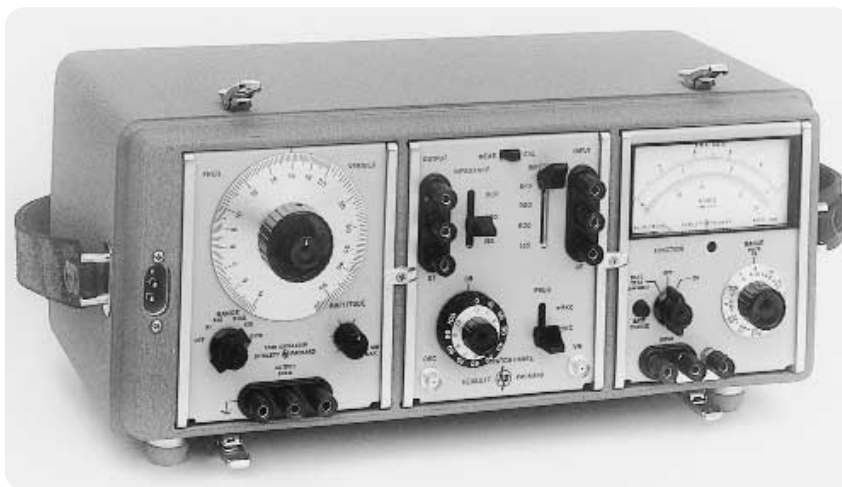
The 3550A frequency response test set could qualify and troubleshoot twisted-pair cables.
