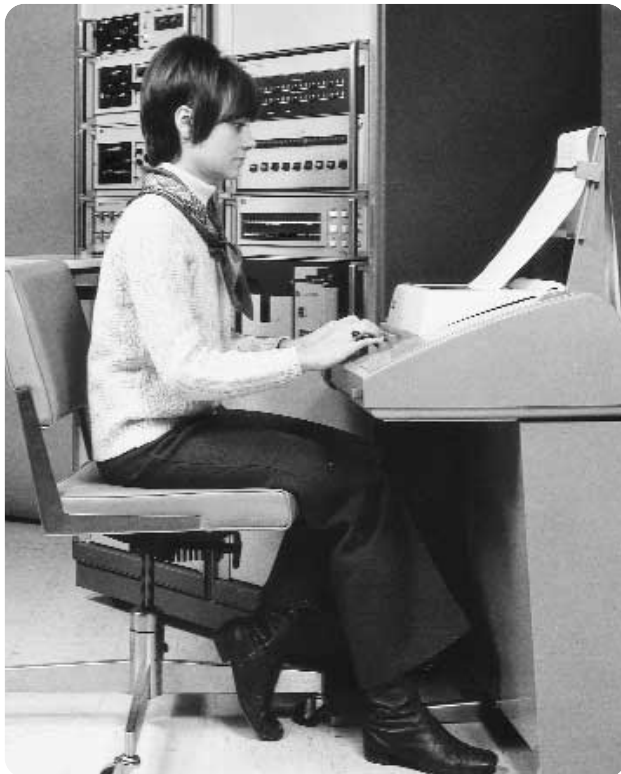
The 8580A automatic spectrum analyzer gathered data for managing satellite communications.
