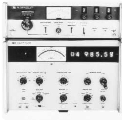
The 312A wave analyzer and 313A tracking oscillator were diagnostic tools for multiplexed cable.
