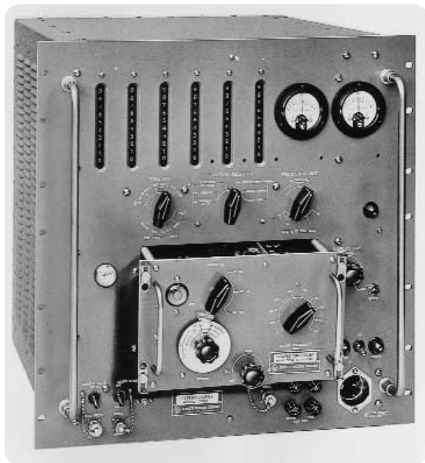
The 524 frequency counter established HP as a leader in electronic counting.
