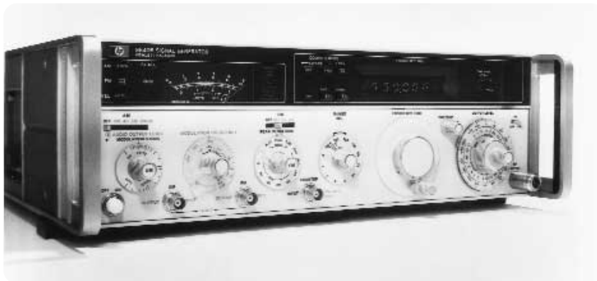
The 8604B VHF signal generator featured built-in phase locking and a 550 MHz counter for high-performance AM and FM signal testing.
