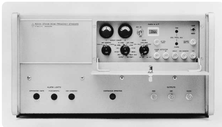
The 5060A cesium beam standard was used to set the world’s clocks.
