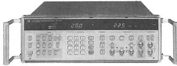
The 3708A gave engineers an accurate way to assess the performance of microwave radio and satellite modem systems.
