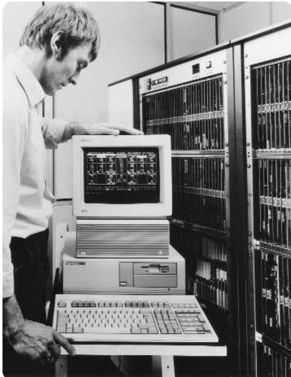
The 37900A signaling test set sped troubleshooting of SS7 networks.
