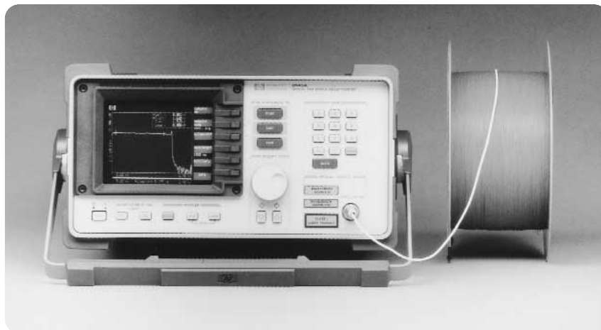
The 8541A OTDR helped engineers characterize long lines of fiber.
