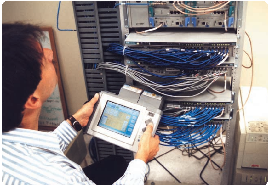
Agilent's tablet-based Service Advisor, part of the Telecom Toolkit, reflects the industry's increasing desire for modular, handheld, multi-format test instruments.
