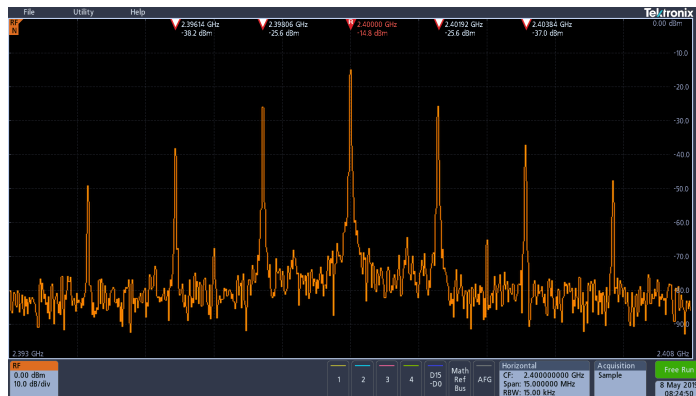
Automated peak markers identify critical information at a glance. As shown here, the five highest amplitude peaks that meet the threshold and excursion criteria are automatically marked along with each peak's frequency and amplitude.
