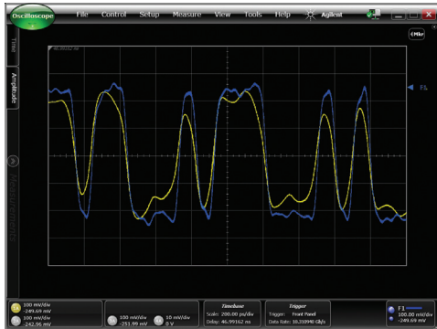
High-fidelity waveform characterization (Yellow: raw trace, Blue: de-embedded waveform)
