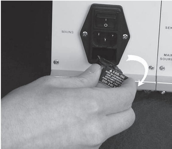
Picture 2–6: Fix the drawer to the input connector assembly
