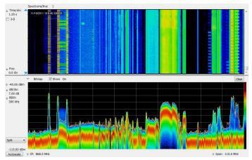
DPX Spectrograms provide gap-free spectral monitoring for up to days at a time. 60,000 traces can be recorded and reviewed, with resolution per line adjustable from 110 µs to 6400 s.
