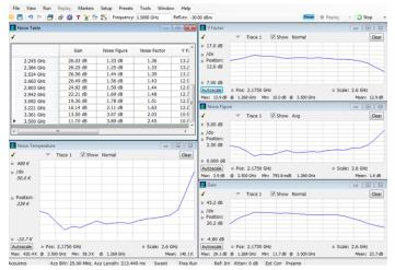
Noise Figure and Gain measurements (Option 14) help you to quickly and easily measure your device using the RTSA and a noise source. This image shows the measurement summary table with graphs of noise temperature, gain, noise figure and Y-
