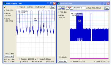
Swept DPX combines the revolutionary DPX Density™ Trigger with the ability to trigger on runt pulses and apply time qualification to any trigger. The runt trigger seen here can be used to track down nonconforming pulses in a pulse train, greatly reducing time to insight. Time qualification can be used to separate ranging pulses from higher resolution pulses in a radar signal, or trigger only on signals that remain on longer than a specified time
