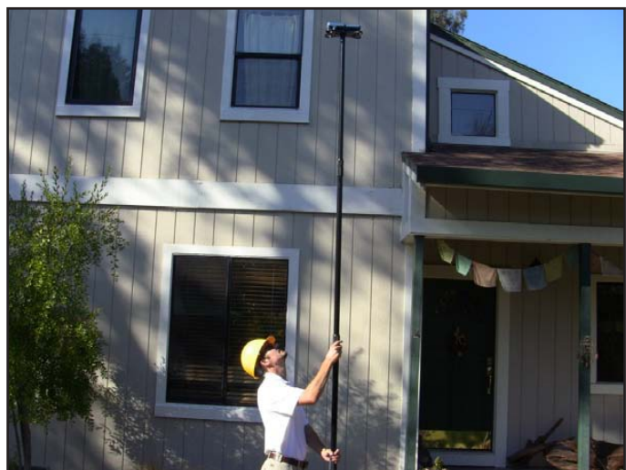
Extension kit enables rooftop measurements from ground level.
