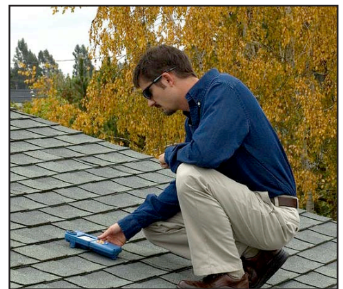
Measuring roof pitch is now integrated into the SunEye 210. Simply lay it on the roof or module and read tilt and heading.
