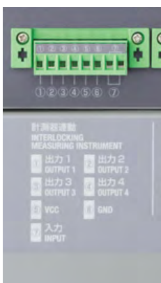
Instrumentation interlock terminals
