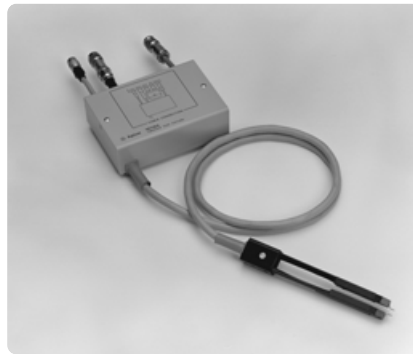
Agilent 16118A tweezer test fixture Tweezer test fixture for easy testing for chip components. Maximum applied voltage: 100 Vdc. Applicable measurement range: \leq 1 \times 10^{11} \Omega (typical). For 4339B only.
