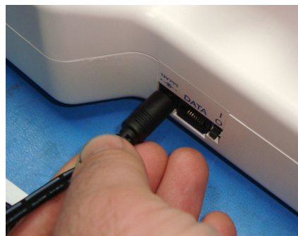
Figure 3-8 Inserting DC Power Plug.
