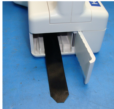
Figure 3-2 Pull Battery Release Ribbon Out
