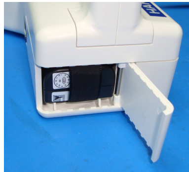
Figure 3-4 Tuck Battery Release Ribbon
