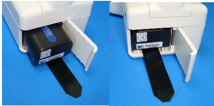
Figure 3-3 Insert Battery into Battery Compartment
