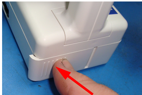
Figure 3-5 Close the Battery Compartment Door
