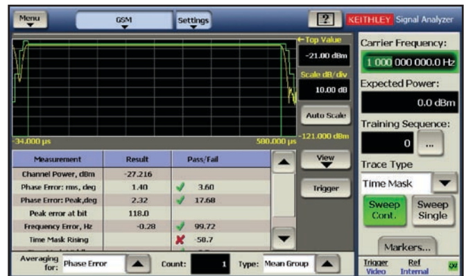
Measure the key parameters of GSM and EDGE signals quickly and easily with the Model 2820-GSM option. The GSM time mask is shown here, along with the results of the signal measurement.
