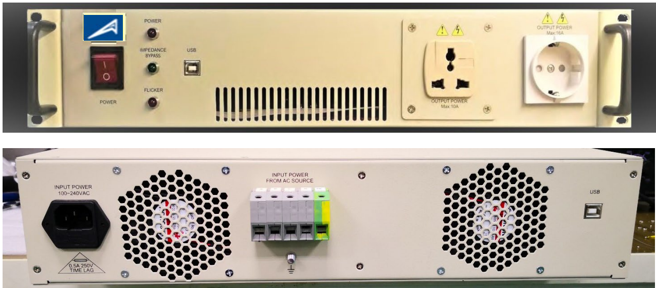
Figure 6 The 19” form factor HFA-1/3 front & rear panel
