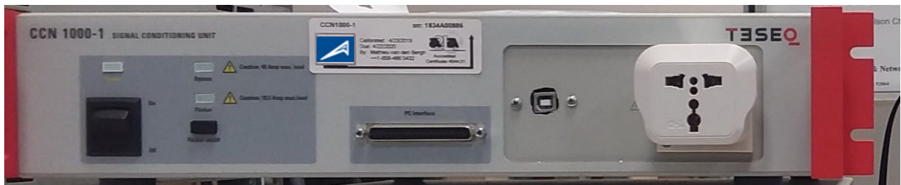
Figure 9 CCN1000-1 upgraded to HFA-1-16 (note the added USB plug on the front)
