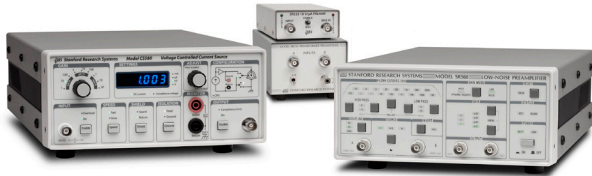
SRS current source and several SRS preamplifiers
