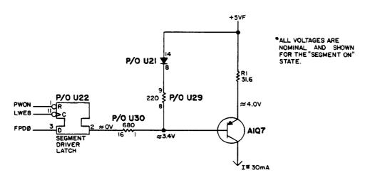
Figure 8-7. Typical Segment Driver Schematic
