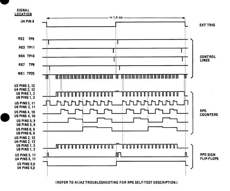
Figure 8-15. RPG Interface Timing Diagram
