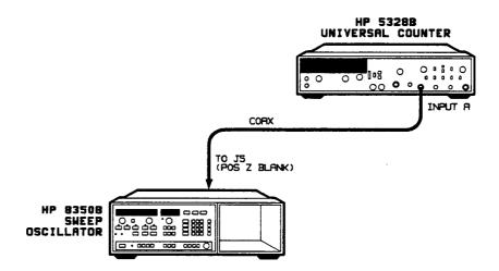
Figure 5-8. Sweep Time Adjustments Setup
