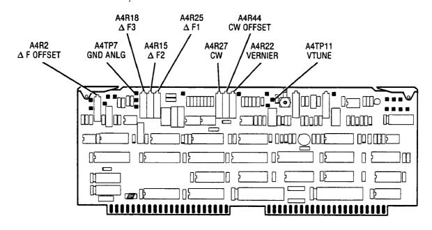
Figure 5-15. Location of Frequency Control Adjustments.
