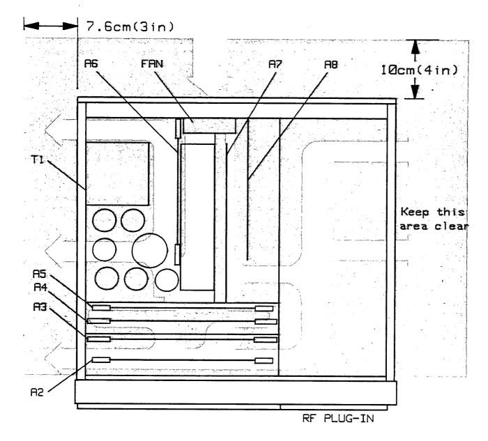
Figure 2-8. HP 8350B Ventilation Clearances Airflow
