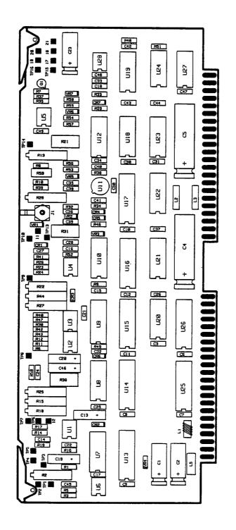
Figure 8-30. A4 Scaling and Marker Component Location Diagram
