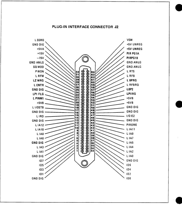
Figure 8-55. Interface Signals on Connector J2
