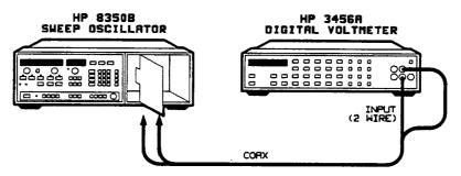
Figure 4-1. Power Supply Test Setup
