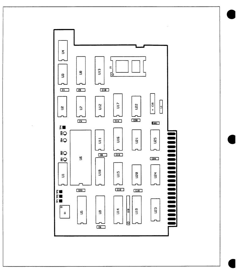
Figure 8-49. A8 HP-IB Interface Component Location Diagram
