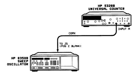
Figure 5-12. Sweep Retrace Time Adjustments Setup
