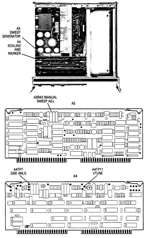
Figure 5-11. Location of Manual Sweep Adjustment.
