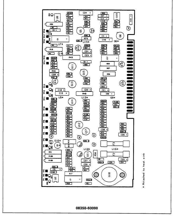
Figure 8-44. A7 Regulator Component Location Diagram
