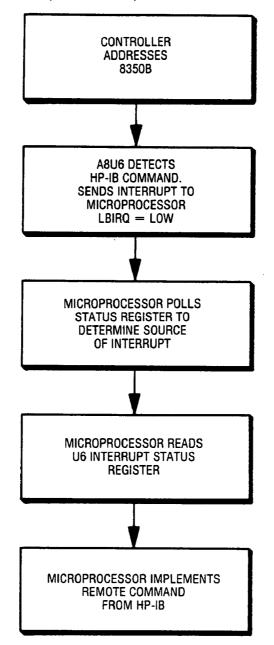
Figure 8-46. HP-IB Interrupt Flow Diagram
