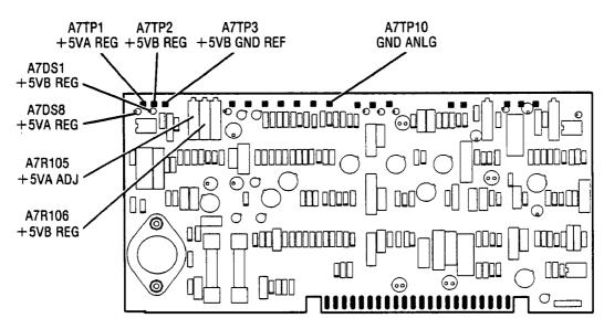
Figure 5-5. Location of +5VA, and +5VB Power Supply Adjustments
