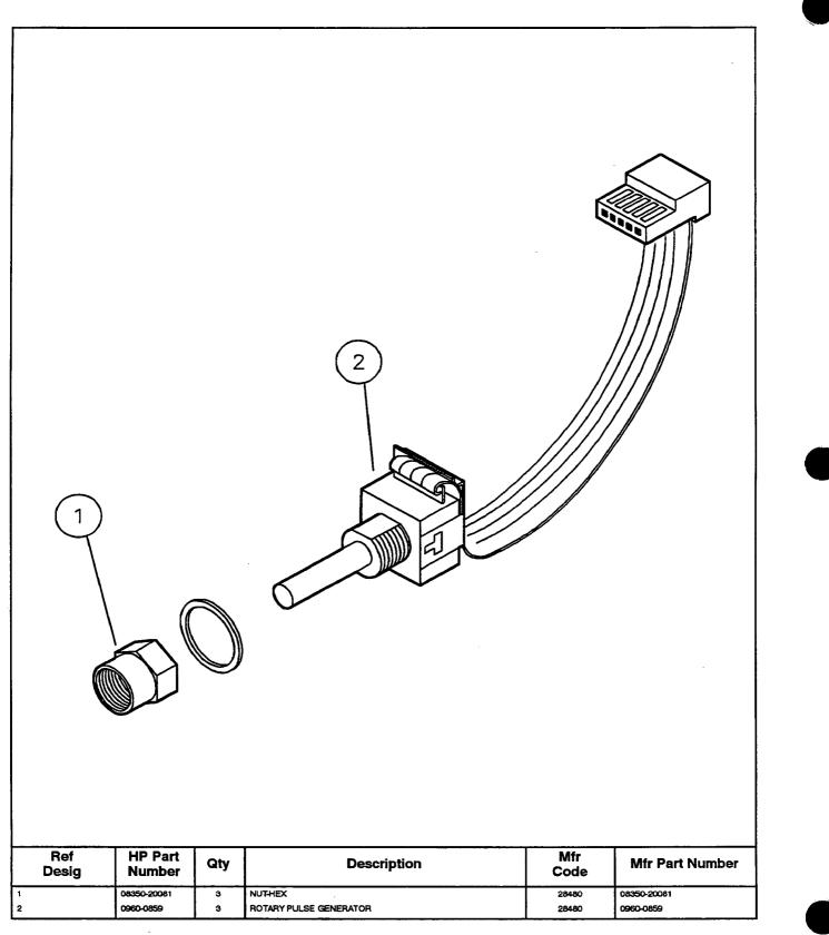
Figure 6-1. Rotary Pulse Generator (RPG), Parts Identification
