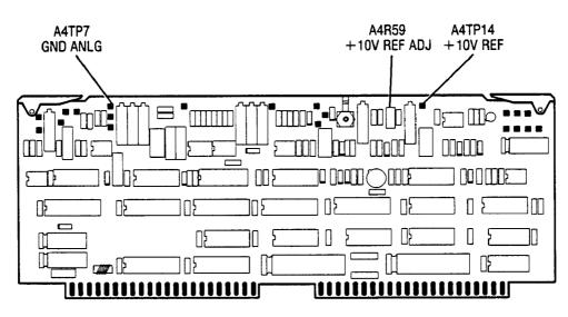
Figure 5-7. Location of +10V REF DAC Power Supply Adjustments
