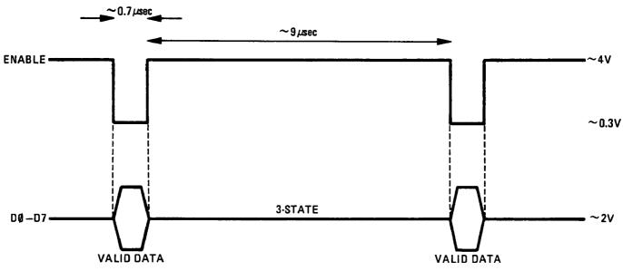
Figure 8-4. Hex Addressed Fast Read - Timing Diagram
