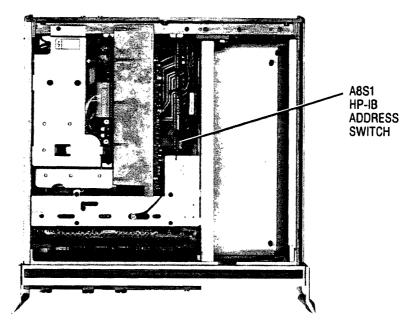
Figure 2-2. Location of A8S1 HP-IB Address Switch
