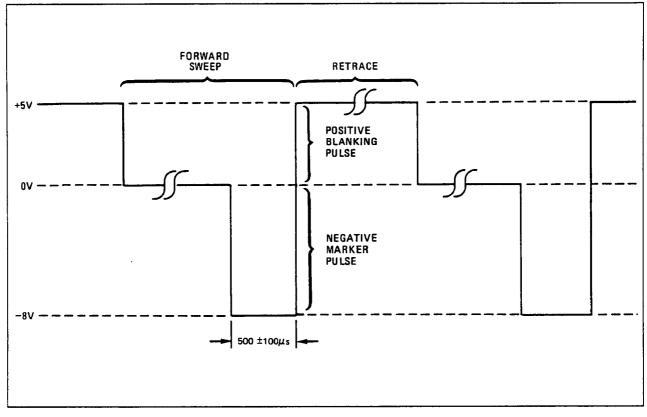
Figure 5-17. Marker DAC Adjustment Waveform
