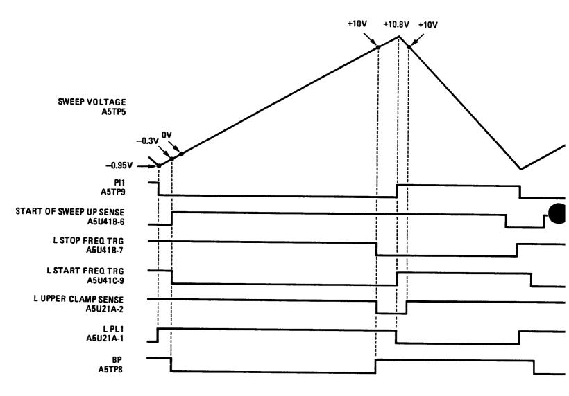
Figure 8-36. Sweep Ramp Status Timing Diagram
