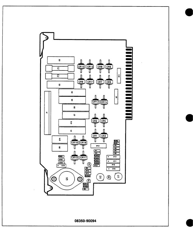
Figure 8-42. A6 Rectifier Component Location Diagram
