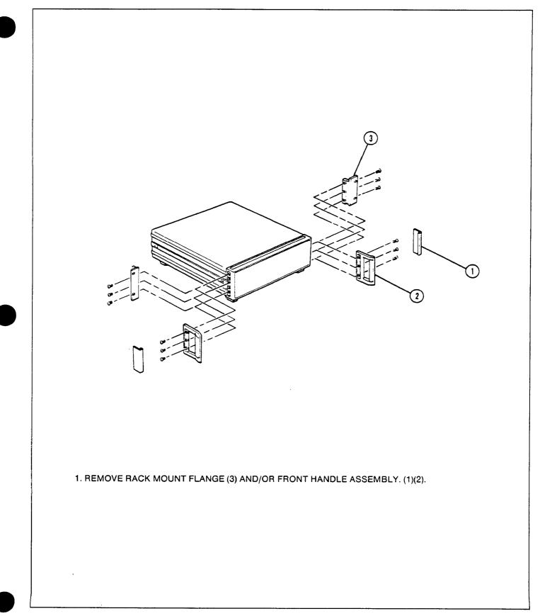
Figure 2-13. Preparation of Instrument for Shipment
