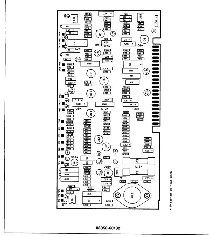
Figure 8-44. A7 Regulator Component Location Diagram
