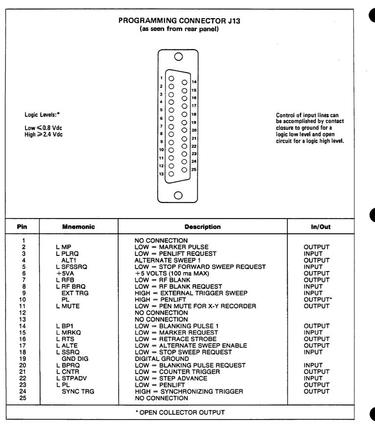
Figure 2-7. Programming Connector Signals and Pin Configuration
