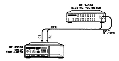
Figure 5-4. +5VA/B Power Supply Adjustment Setup
