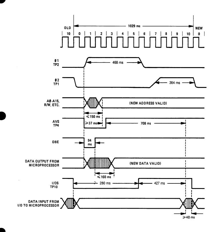
Figure 8-20. A3 Microprocessor Read/Write Timing Diagram
