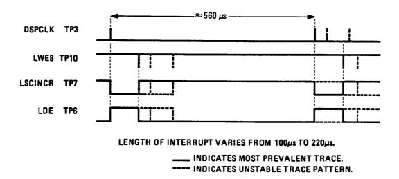
Figure 8-14. Front Panel Interrupt Timing Diagram
