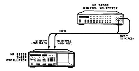
Figure 5-6. +10V REF DAC Power Supply Adjustment Setup
