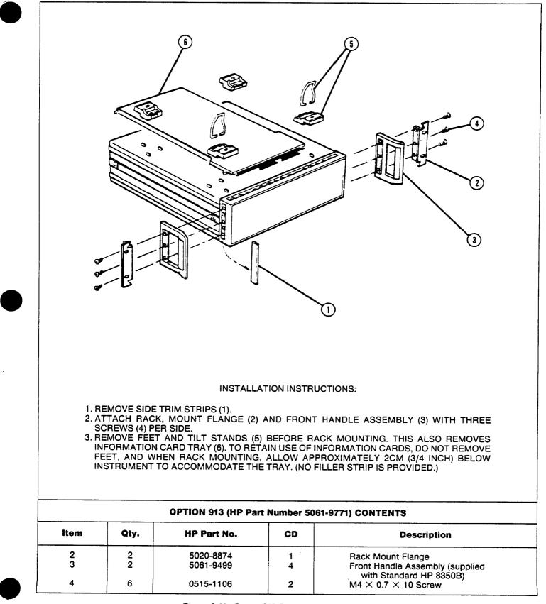
Figure 2-11. Option 913 Rack Mount Kit with Handles
