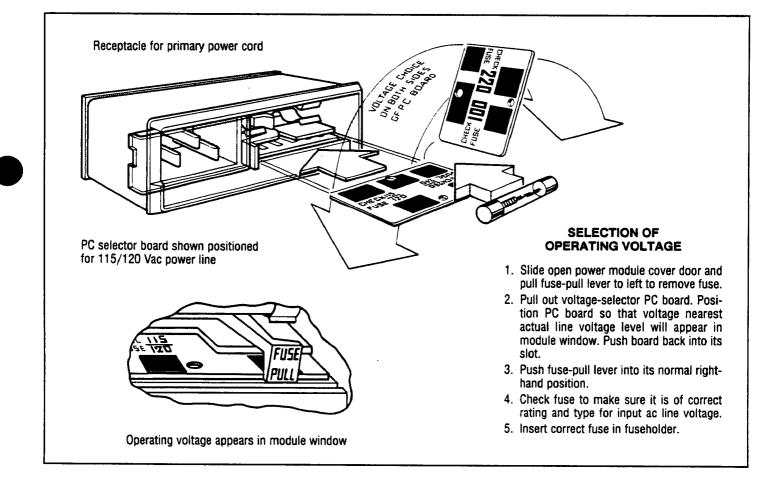
Figure 2-1. Power Line Module
