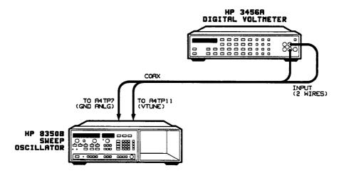
Figure 5-14. Frequency Control Adjustments Setup
