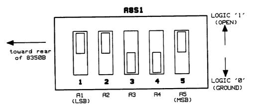
Figure 2-3. A8S1 HP-IB Address Switch
