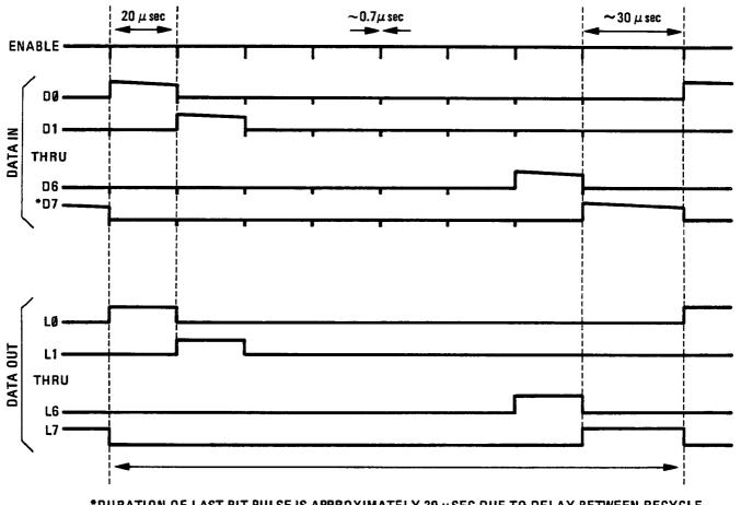
\*DURATION OF LAST BIT PULSE IS APPROXIMATELY 30  $\mu\,\text{SEC}$  DUE to delay between recycle.
