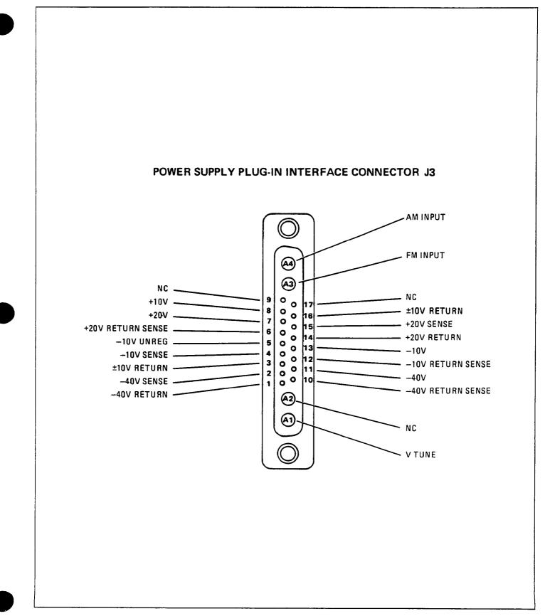
Figure 8-54. Interface Signals on Connector J3
