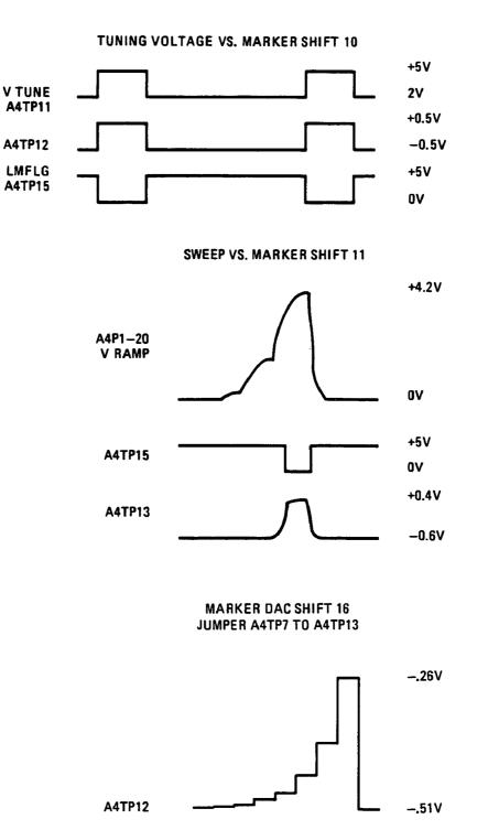
Figure 8-28. Operator Initiated Self Tests (1 of 2)
