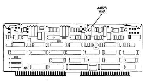
Figure 5-18. Location of Marker DAC Adjustment
