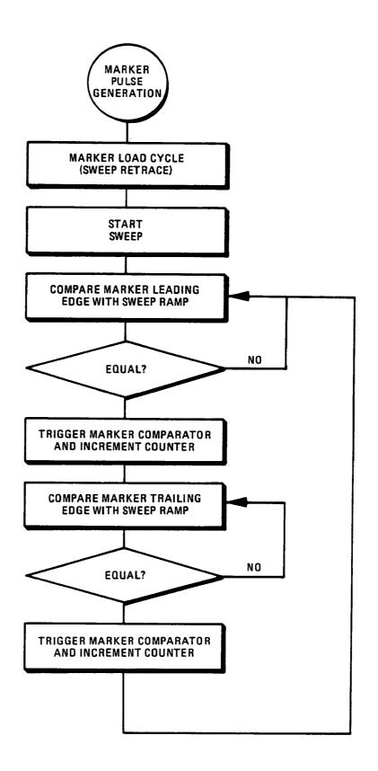
Figure 8-24. Marker Pulse Generation, Flow Diagram
