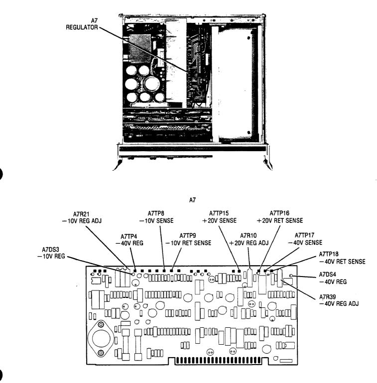
Figure 5-2. Location of +20V, -40V, and -10V Power Supply Adjustments
