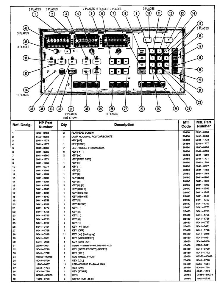
Figure 6-4. Sub Panel, Parts Identification
