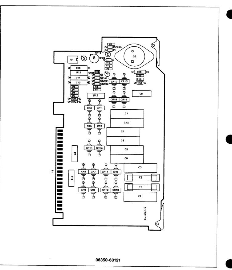
Figure 8-42. A6 Rectifier Component Location Diagram
