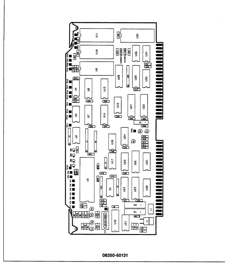
Figure 8-22. A3 Microprocessor Component Location Diagram
