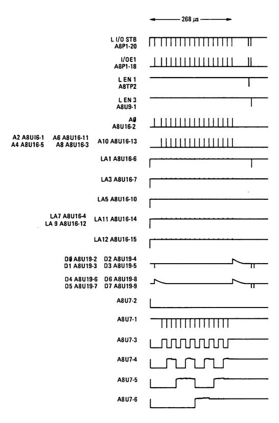
Figure 8-48. Instrument Bus Self Test, Timing Diagram (1 of 2)
