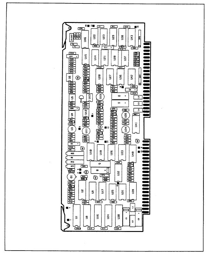
Figure 8-37. A5 Sweep Generator Component Location Diagram
