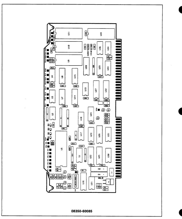
Figure 8-22. A3 Microprocessor Component Location Diagram
