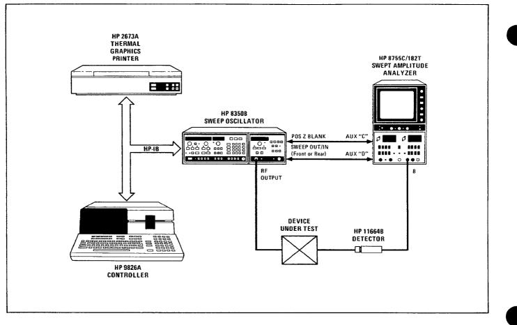
Figure 2. Equipment Setup
