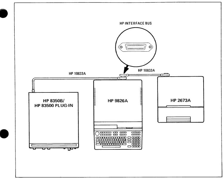
Figure 1. System Connection
