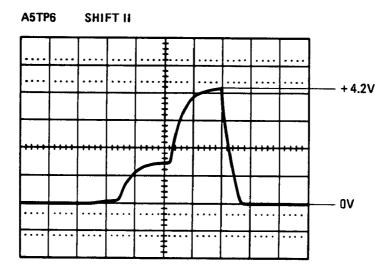
Figure 8-34. Sweep Voltage Waveforms for Sweep versus Marker Self Test
