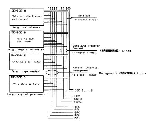
Figure 3-5. Interface Connections and Bus Structure
