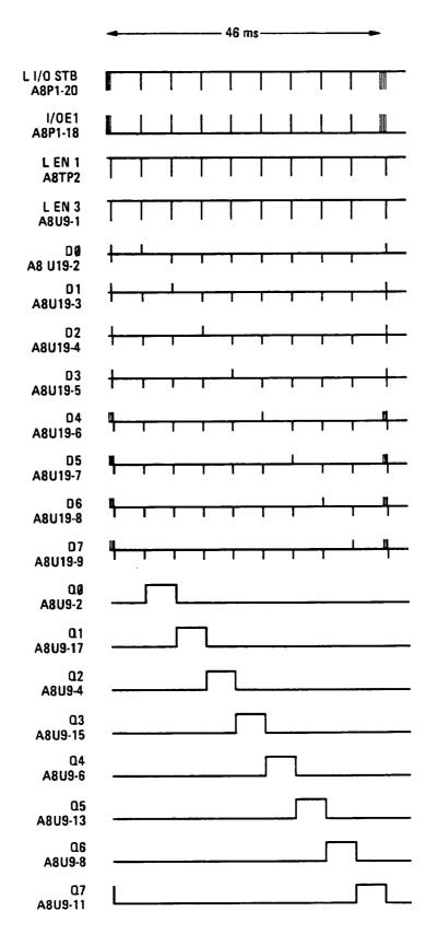
Figure 8-48. Instrument Bus Self Test, Timing Diagram (2 of 2)
