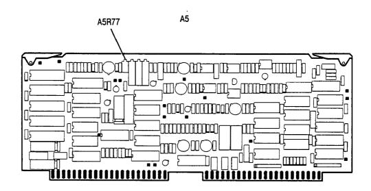
Figure 5-13. Location of Sweep Retrace Time Adjustments.
