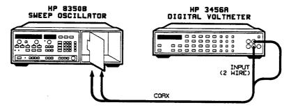
Figure 4-2. Tuning Voltage Check Test Setup
