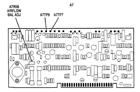
Figure 5-3. Location of AIRFLOW BALance Adjustment
