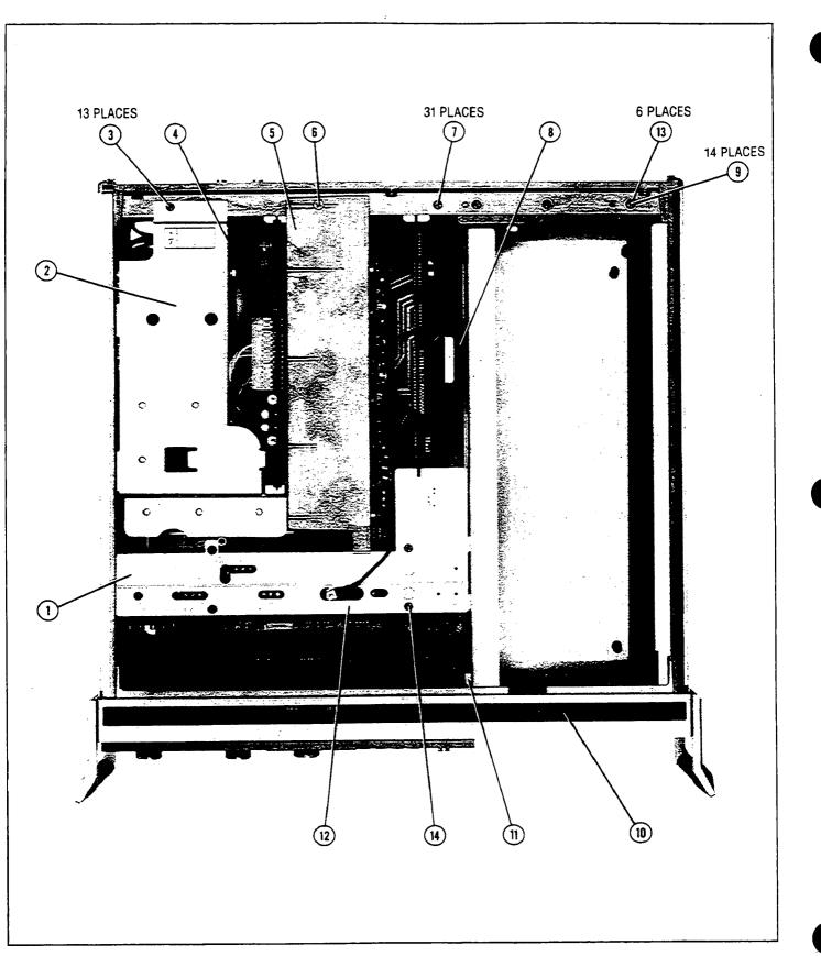
Figure 6-5. Top View with Covers, Parts Identification (1 of 2)
