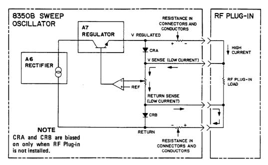
Figure 8-39. Typical Post Regulated Power Supply, Simplified Schematic
