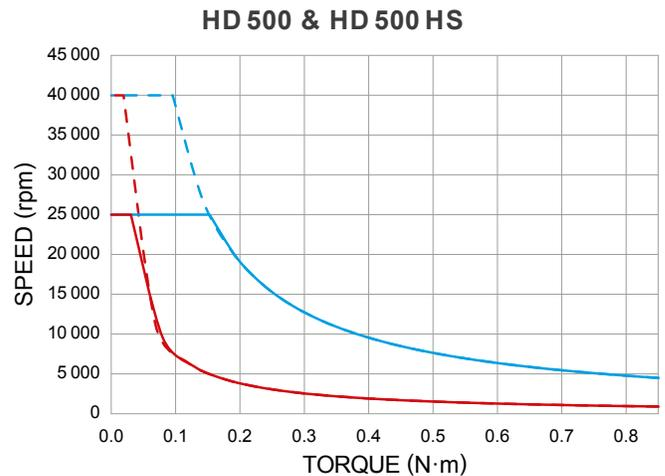
The power absorption curves represent the maximum power (heat) that the dynamometer can dissipate over time.
