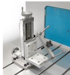
Positioning and alignment have a great influence on the measured parameters (friction torque). MAGTROL strongly recommends a support specifically dedicated to the products to be tested to ensure the best positioning tolerances in X-Y, and its repeatability.
