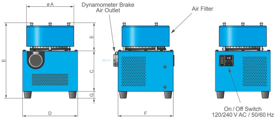
Allow approximately 6 in to 8 in (152 mm to 203 mm) between rear of dynamometer base plate and blower for connection hardware. Required hardware is supplied with the dynamometer.
