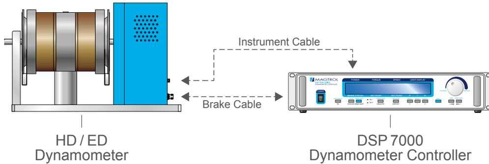
Fig. 2: Dynamometer with DSP 7000 Dynamometer Controller
