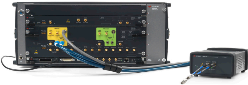
Figure 3. The remote head M8057A is required for each channel and is required for NRZ and PAM-4 signals. It contains an adjustable gain amplifier without re-timer. Users can select NRZ or PAM-4 coding and de-emphasis taps settings from the user interface with no need to reconnect cables. The cable between the remote head and the module is 0.85 m long. This allows positioning the remote head closely to the test board for the device under test.
